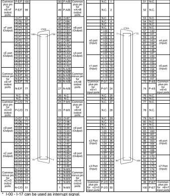
I-00 - I-77 64 channels input signal. Connect output signals from the external device to
