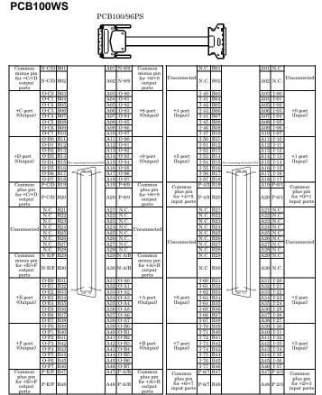
Pin assignments for connecting to the PCB100/96PS or
