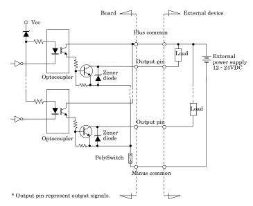
The output circuits of interface blocks of the PIO-32/32L(PCI)H and PO-64L(PCI)H are illustrated in Figure 3.7. The signal output section is an opto-coupler isolated, open-collector output (current sink type). Driving the output section requires an external power supply.
