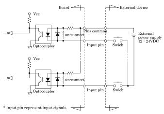
The input circuits of interface blocks of the PIO-32/32L(PCI)H and PI-64L(PCI)H are illustrated in Figure 3.5. The signal inputs are isolated by opto-couplers (ready to accept current sinking output signals). The board therefore requires an external power supply to drive the inputs. The power requirement for each input pin is about 5.1 mA at 24 VDC (about 2.6 mA at 12 VDC).
