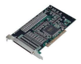
Digital Input Board with Opto-Isolation for PCI **PI-64L(PCI)H**
