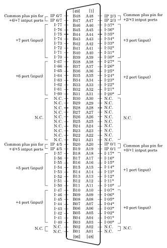
\* I·00 · I·37 can be used as interrupt signal. The numbers in square brackets [ ] are pin numbers designated by HONDA TSUSHIN KOGYO CO., LTD.
